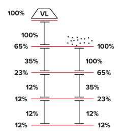
To maintain an adequate margin of safety, three levels of back props are required to ensure the increased floor loads remain within safe limits.
